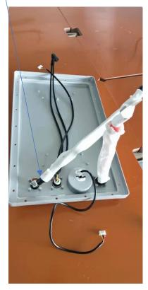
18. Connect the positive cable from lid to the positive pole of cell pack. Connect the negative cable from lid to the P- of BMS, using
