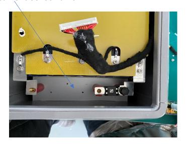
10. take off the power cables from current sensor unit.
