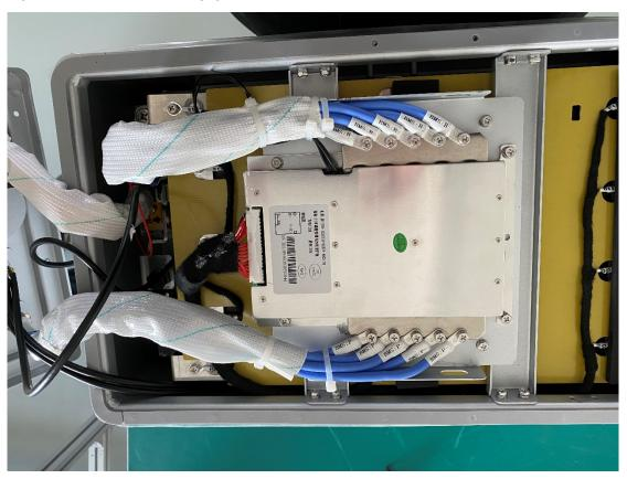
2. Unplug the cell volt connector from XK BMS
