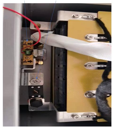
16. Bring the B- power cable from current sensor, connect to the B- of BMS, using M5\*10 screws. Please place the new seal strip around the case. (This power cable will go through center of cooling pad of BMS, please use tape to fix it.)
