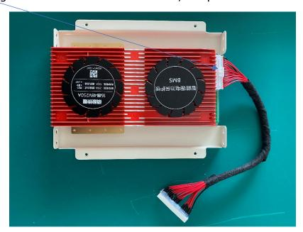
14. Install Daly BMS to metal case, please note the cell volt wire connector should be go through under the support frame.
