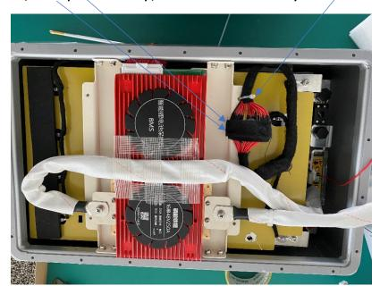
21. Connect two connectors to current sensor, use glue to fix it.
