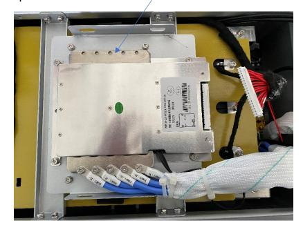
4. Take out the temperature sensor. <u>must wrap the terminal of power cable (from P- port of BMS in last step) to avoid short circuit.</u>
