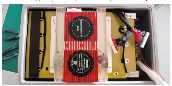
15. Install current sensor and fuse unit.
